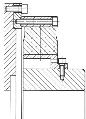
Series SR drop-out-type, element is comprised of 4 segments, for torque range of 20000 to 60000 Nm.
