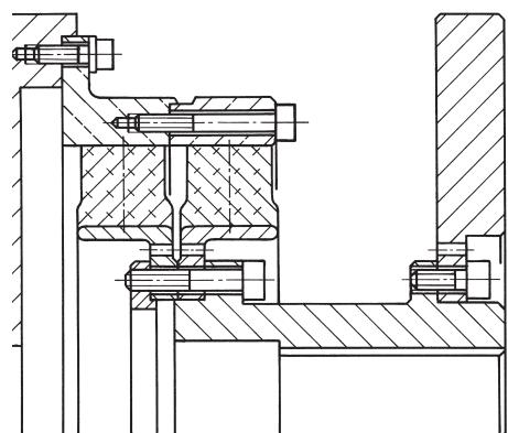
CM-8000-SDE, drop-out type, with special hub and additional inertia.
