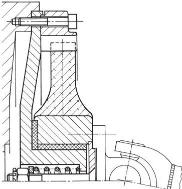
As intermediate coupling for cardan shafts.
