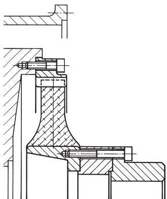
Drop-out-type, with spacer for deep fly-wheels or flywheel housing.
