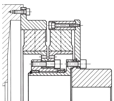
Drop-out-type, with 2 elements in line, giving double torsional elasticity, half torsional stiffness.
