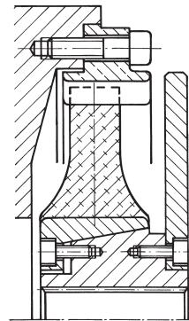
with 3 special features: a) outer ring protrudes into flywheel for short overall length. b) inner hub elongated towards engine for longer spline engagement. c) with secondary extra inertia for low resonance speeds.
