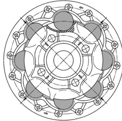
The CENTAFLEX-R is a simple robust ROLLER coupling with a progressive torsional characterisation. Ideal for boat drives, providing a very low stiffness at low torque (& speed) which shifts the torsional resonance below idle speed and prevents gearhammer (gear chatter).
