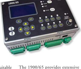
The 1900/65 provides extensive capabilities: eight input channels; six configurable alarm relays; four 4-20 mA outputs; buffered output facilities for easy connection to portable diagnostic instruments; Microsoft® Windows®-based configuration software; an optional easy-to-read display that can be mounted locally or up to 75 meters (250 feet) away; and an optional IP65-rated weatherproof housing (or door for panel-mount applications).
